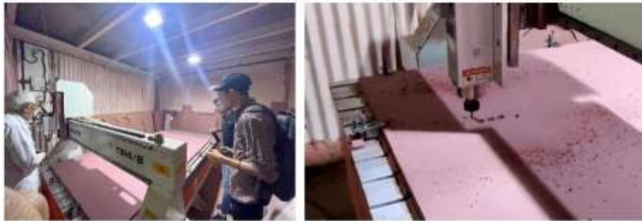
CNC cutting process for the MDF board base
